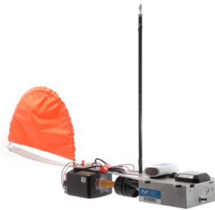
The miniPCS in field configuration. The air containing particles is pulled through the probe volume by the pump at the rear. A removable filter ahead of the pump is used collect particle samples.
