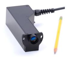
The microPro, the size of a small flashlight, is self contained and permanently aligned; no calibration required by the user. The probe contains a miniLDV, micro translation stage, and receiving optics. MSE will provide custom attachment hardware designed for your flow facility. Below is an example of an attachment for circular pipes.
