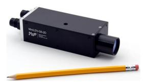
The 2D miniLDV System with 50 to 240 mm standoff is extremely compact, self contained, and permanently aligned; no calibration or alignment by the user is required. The probe contains two high power diode lasers, miniature beam shaping optics, and receiving and detection optics.
